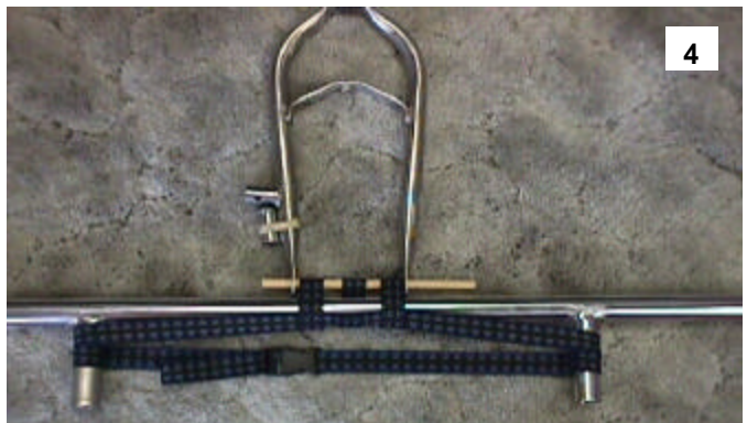
Picture 3 - close-up of 'Jordan Air' hitch assembly
